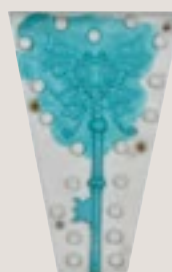
STEP 3 Rubber Mould with Wax Inside
